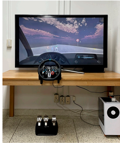
Figure 1. An image of the experimental setup. The steering wheel and the accelerator pedals were aligned to the center lines of the HUD and HDD in the display.
